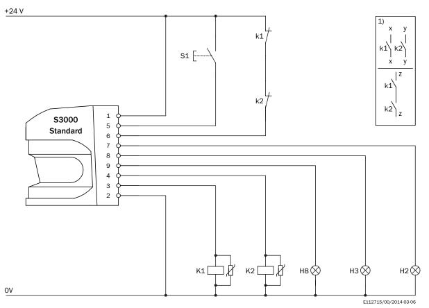
S3000 Standard in conjunction with relays/contactors
