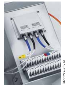
Fig. 5/148 Communication interfaces in a sloped case in a surface-mounting housing
