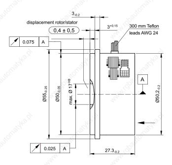
Inner diameter stator = 33.470 min. Outer diameter rotor = 32.735 max.
