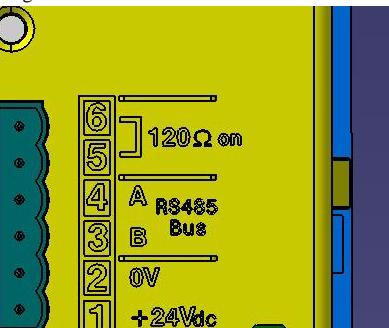
In case of communication via the Internal bus, the HMI030 unit must be configured in Master mode. Infact, at start-up, if in Master mode, the HMI030 unit polls alternatively the Modbus and the Internal bus, and starts the data transmission on the bus that first responses affirmatively; to the contrary (that's if in Slave mode), the HMI030 unit tries to communicate exclusively via Modbus.
