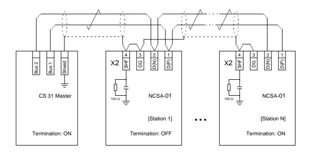
Figure 4-4 CS 31 bus cable connection.
