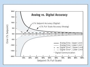
At 10% setpoint, digital MFCs are ten times more accurate than analog models. (Accuracy chart reflects primary standard calibration option.)\*\*
