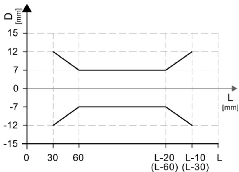
Measurement deviation D at the limits of the active rod range
