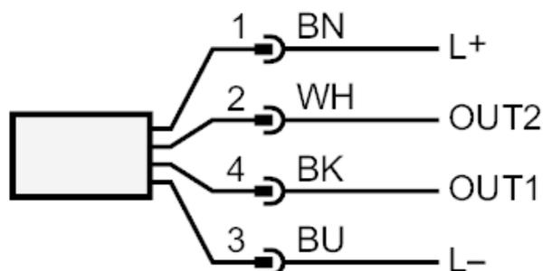
OUT1: switching output or IO-Link
